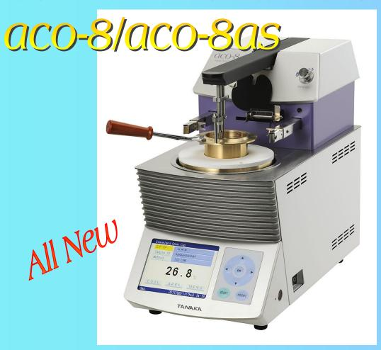
Model aco-8 and aco-8 asphalt version are the automated Cleveland Open Cup flash point tester from Tanaka. Based on 45 years experience of manufacturing the automated flash point testers, innovative 8<sup>th</sup> generation series has been released. The theme of 8th generation is "Ergonomic, Versatile and Premium".
