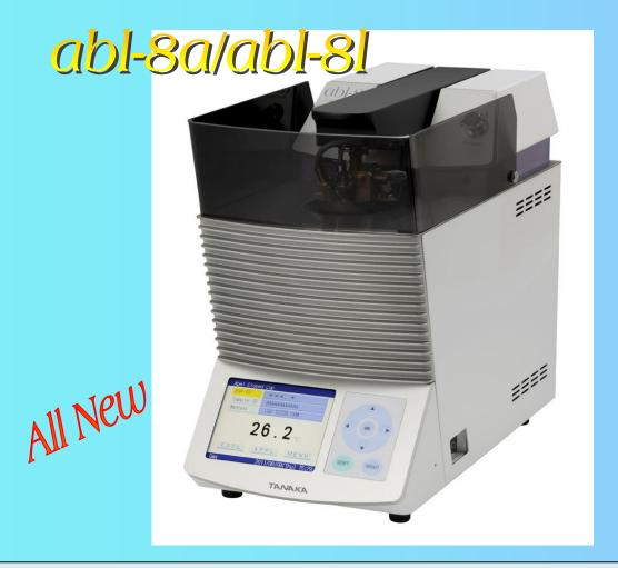
Model abl-8 series is the automated Abel Closed Cup flash point tester from Tanaka. Based on 45 years experience of manufacturing the automated flash point testers, innovative 8th generation series has been released. The theme of 8th generation is "Ergonomic, Versatile and Premium".
